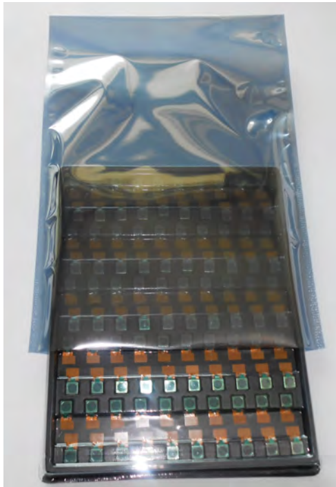
Put Tray into Anti-Static Bag
